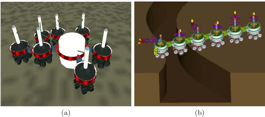
Fig. 1. Graphic visualisation of how the rigid gripper can be used to connect in a secure way s-bots among themselves so that they form a swarm-bot for (a) retrieving heavy objects or (b) passing over holes.
