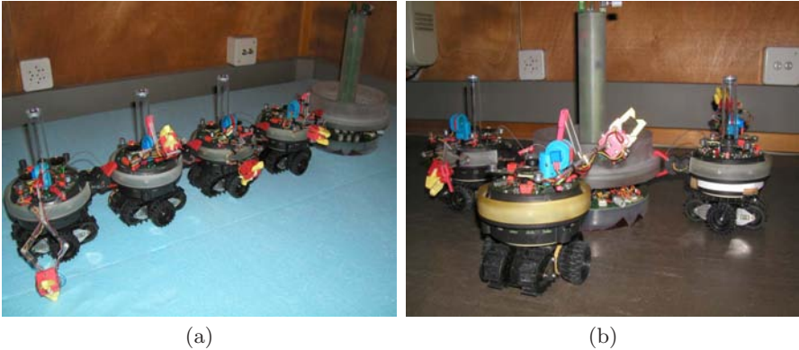
Fig. 3. Pictures of s-bots transporting an object that can not be moved by a single s-bot . (a) A swarm-bot comprising four s-bots pulls an object. (b) Three s-bots pull/push an object to which they are directly attached.
