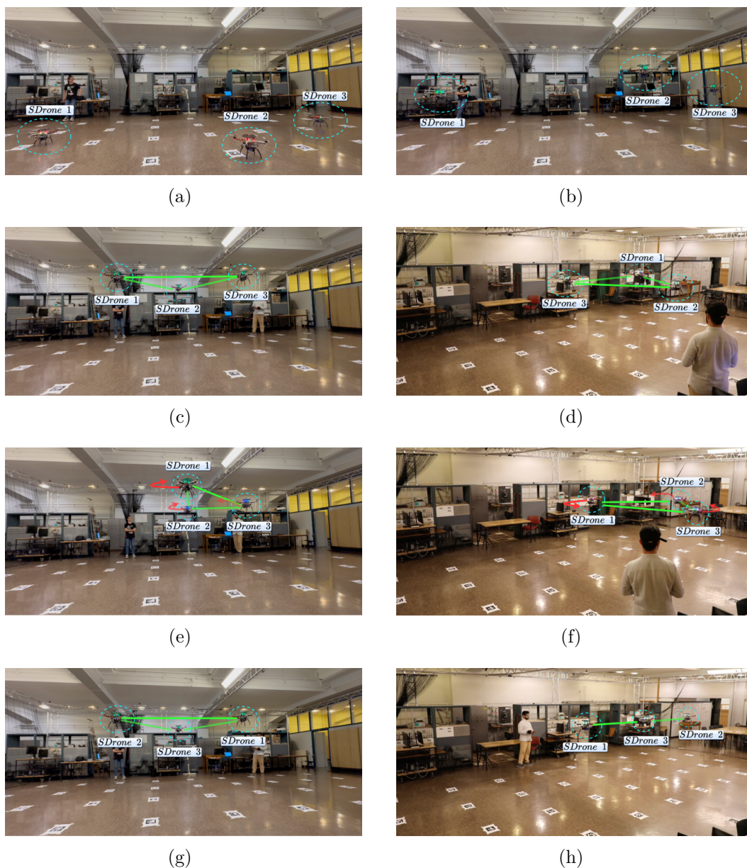
Figure 3.21: Demonstration of multi-UAV flight in a dynamic formation: (a) Initial random placement of the three UAVs. (b) Take-off procedure. (c) Establishment of a triangle formation. (d) Alternative perspective of the established triangle formation. (e) Start of formation rotation. (f) UAVs in rotation. (g) Completion of the rotation. (h) Final reconfiguration transitioning from triangular to linear formation. (Reprinted from (Oğuz et al., 2024).)
