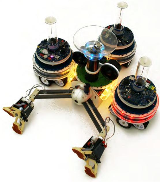
Figure 4.19: A picture that shows three foot-bots attached to the object to carry, in this case another robot of a different kind. See [Dorigo et al. \(2012\)](#) for more information on the use of this robot assemble.
