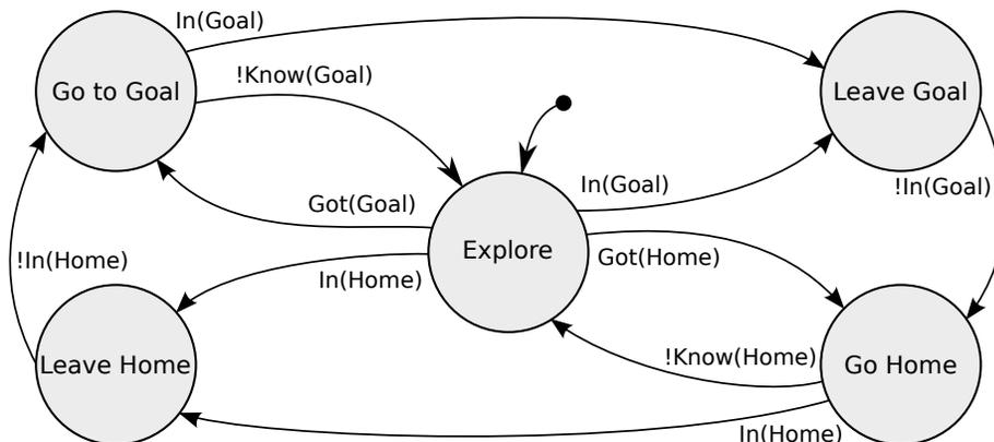
Figure 3.1: Robot’s finite-state automaton. The circles define the states while the arrows define the transitions.  $In(Area)$ ,  $Area \in \{Home, Goal\}$ , is true when the robot senses the grey level of the area,  $Know(Area)$  is true when the robot knows the position of the area,  $Got(Area)$  is true when it just gets this estimation. The robots start in the *Explore* state.
