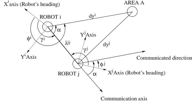
Figure 2.1: Diagram of the transformation of the shared position of area A between the frame of reference of robot  $i$  (emitting) and robot  $j$  (receiving), reprinted from Gutiérrez et al. (2009)
