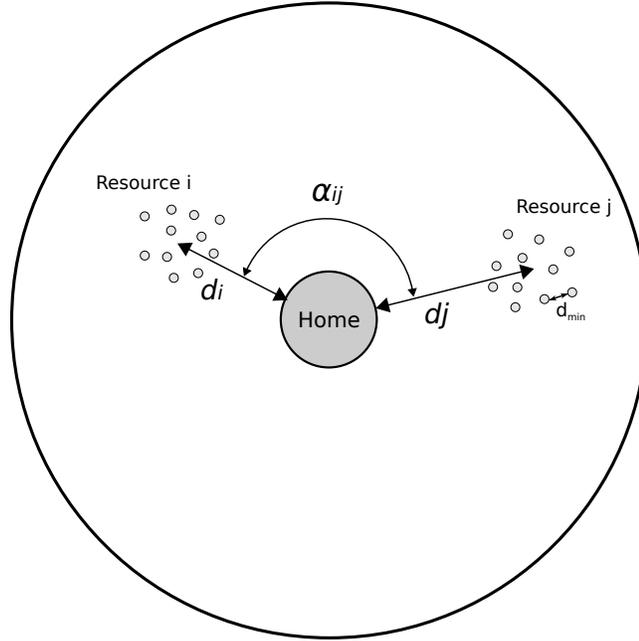
Figure 4.2: Setup of the experimental arena for the exploitation task. The home area is placed in the center of a circular arena of an 11 m radius, surrounded by walls. In this setup, the goals are resources, defined as a Gaussian spread of items with a minimum distance between them of  $d_{min}$  (five times the robots' radius). They are characterised by their distance from home  $d_i, d_j$ , the angles they form with each other  $\alpha_{ij}$  and their respective quality.
