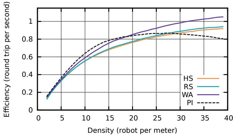
Figure 3.3: Impact of density on navigation efficiency for each mechanism and in the perfect information control condition. Each line is the mean over 100 trials.
