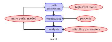
Fig. 7 Overview of the statistical model checking approach
