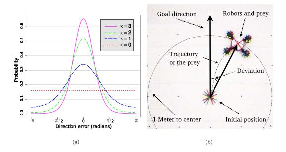
Figure 2: (a) The effect of parameter  $\kappa$  on a von Mises distribution. (b) A snapshot describing the final situation of a successful transport. Note how the deviation of the transport direction from goal direction is measured.
