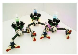
**Figure 4.** Three hand-bots assembled together. The handbot is an autonomous robot capable of climbing vertical structures and manipulating objects. The grasping hands provide basic manipulation abilities. They also enable handbots to physically connect to one another, thus forming larger composite robotic entities.
