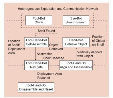
Figure 8. Search-and-retrieval behavioral components. The dotted lines represent information transfer. The solid lines represent handing over of control to another behavioral component. The swarmanoid must initially be launched by executing the heterogeneous exploration and communication network behavioral components, while each execution of the foot-hand-bot disassemble and reset behavior marks the successful return of a single object to the deployment area.
