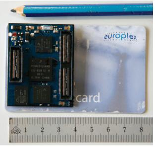
Figure 2. The half-credit-card-size i.MX31 main processor board.
