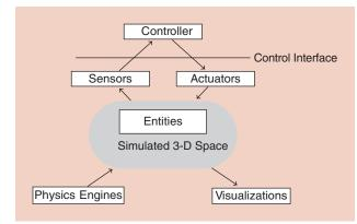
Figure 6. The architecture of the ARGoS simulator.
