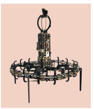
**Figure 5.** The eyebot platform. The eyebot is an autonomous flying robot suited to collective exploration of indoor environments. Eye-bots stay in contact with each other using the range and bearing communication device. The ceiling attachment device allows eye-bots to extend their energy autonomy by powering down their flight systems.
