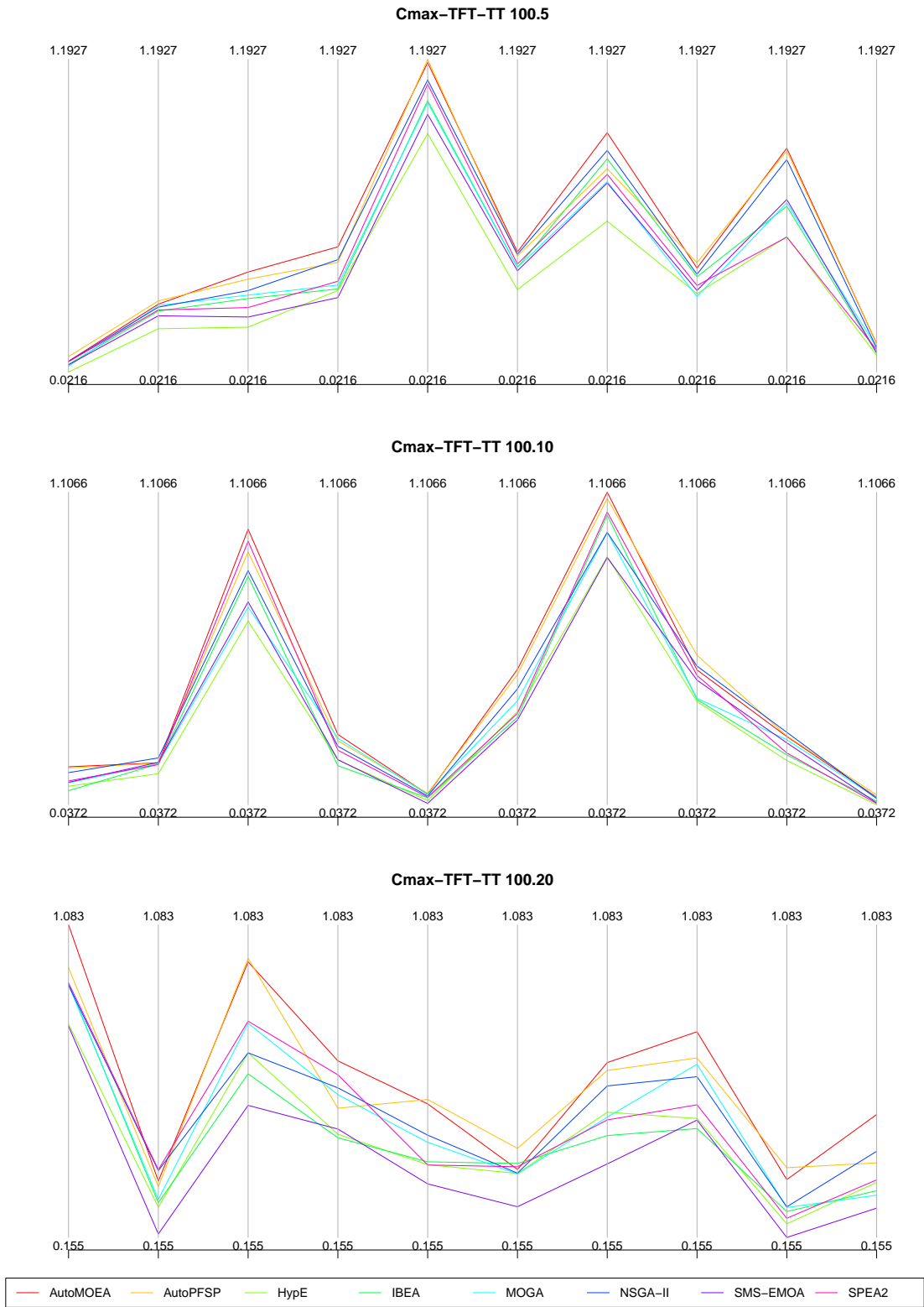
Fig. 15: Average hypervolume over 10 runs on 10 instances with 100 jobs each of Cmax-TFT-TT.
