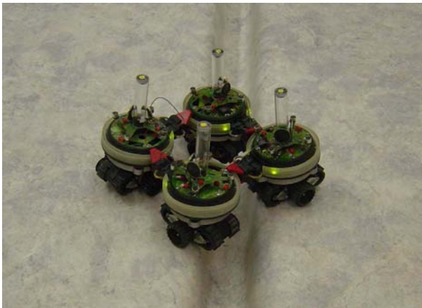
Figure 7. A swarm-bot composed of four s-bots in square formation passing over a trough.
