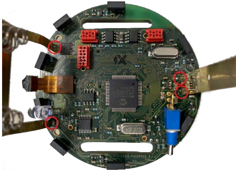
Figure 3: E-puck basic board. The soldering positions of the battery connectors are indicated by red circles.
