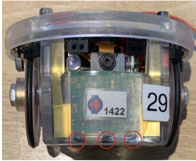
Figure 2: Ground sensor module inserted properly into the e-puck housing. The left, middle, and right ground sensors (indicated by red circles) are settled at the bottom of the housing.
