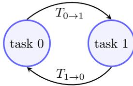
Figure 1: Agent controller as probabilistic finite state machine for the simplistic two-task allocation. Transition conditions  $T_{0 \rightarrow 1}$  and  $T_{1 \rightarrow 0}$  are defined by the respective agent controller type and need to depend on locally measurable features only.
