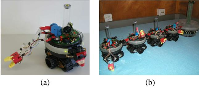
Fig. 1. The swarm-bot concept: (a) a single module called s-bot capable of locomotion and perceiving the environment, (b) a modular robot called *swarm-bot* composed of four s-bots manipulating an object.
