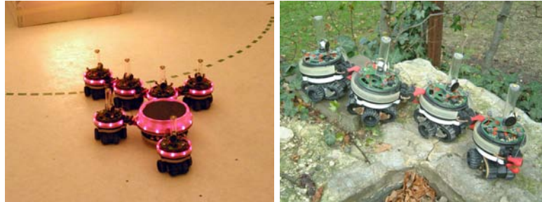
Fig. 2. Left: 6 s-bots, of which 4 in swarm-bot formation, collaborate to transport a heavy object. Right: A 4 s-bots linear swarm-bot moves on rough terrain.
