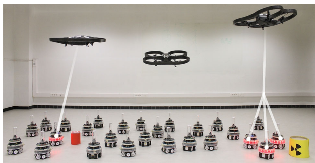
Fig. 1 An illustration of spatially targeted communication. The overlays show the ad-hoc communication links the aerial robots establish to communicate with specific robots on the ground that are situated next to the objects of interest
