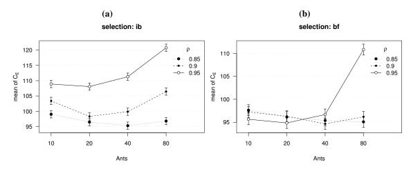
**Figure 6.20:** Interaction between the number of ants and persistence factor  $(\rho)$  in the results of MMAS for the Richmond network.
