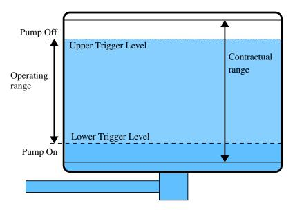
**Figure 3.4:** Trigger levels on a tank.
