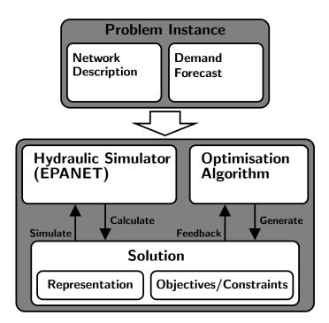
**Figure 2.1:** Schematic diagram of pump scheduling optimisation system.
