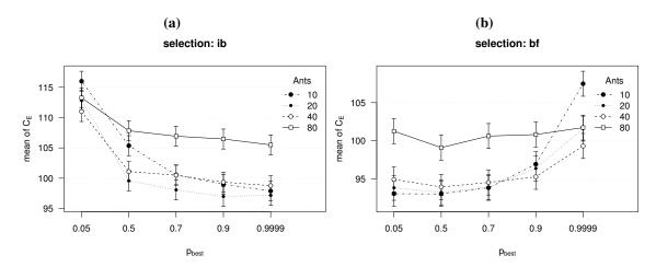
**Figure 6.21:** Interaction between the number of ants and  $p_{\text{best}}$  in the results of MMAS for the Richmond network.
