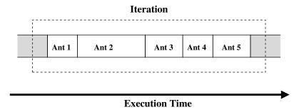
**Figure 6.25:** Sequential evaluation of solutions in ACO.
