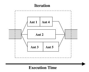
**Figure 6.26:** Parallel evaluation of solutions in ACO.
