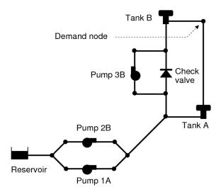
**Figure 2.2:** Vanzyl test network.
