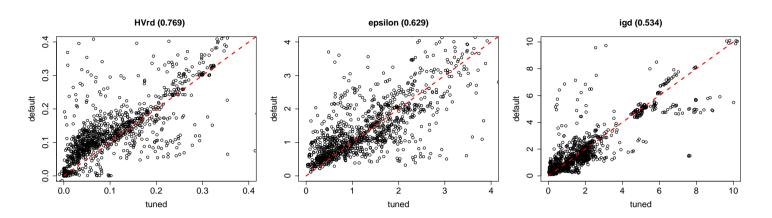
Figure 1: Scatter plots comparing the performance of tuned (*x*-axis) and default (*y*-axis) parameter configurations of MOEAs according to the  $I_H^{rd}$  (left),  $I_{\epsilon+}^1$  (center), and *IGD* (right) metrics. Each point is the mean result of 25 runs of the same MOEA on a particular benchmark problem with the same stopping criterion.
