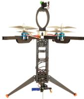
As reference models for the planner nodes, we consider the *eye-bot* robots, that are being developed in the Swarmanoid project (<http://www.swarmanoid.org>). These are small flying robots that can attach to the ceiling, are equipped with a video camera pointing to the floor, and have an infrared system for measuring the relative bearing and distance between two robots and for wireless communications.
