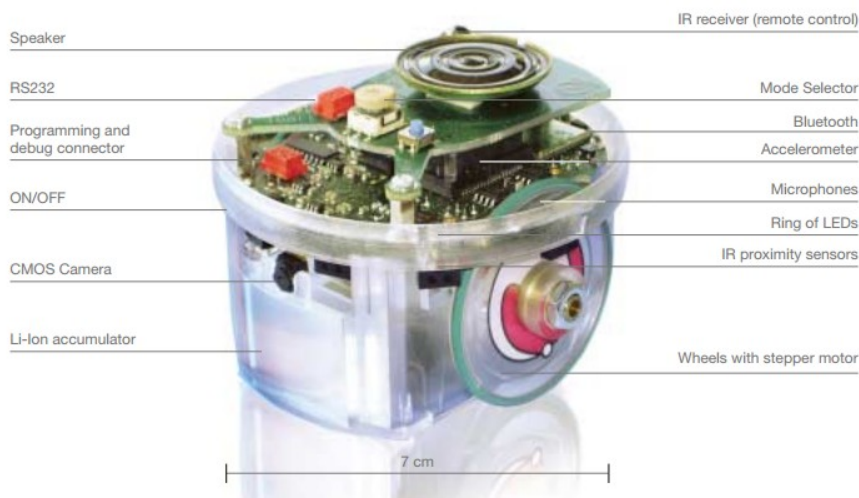
Figure 5: Annotated picture of the e-puck robot. (Courtesy of RoadNarrows )
