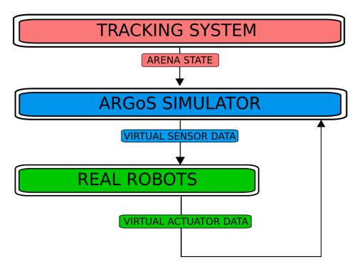
Figure 13: Communication flow in the system
