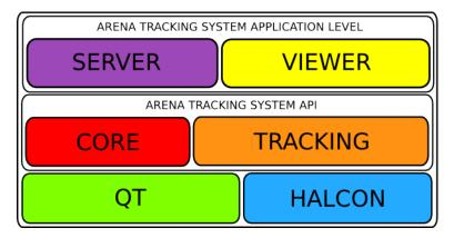
Figure 3: Arena Tracking System Software Architecture
