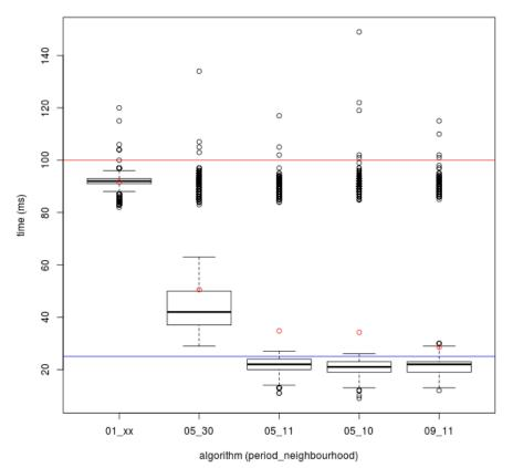
Figure 10: ATS marker detection efficiency in ms. The red line at 100 ms is a required upper bound for efficiency performances. The blue line at 25 ms is an ideal upper bound that allows a four camera experiment to meet the requirement of 100 ms for timestep. The red points represent the average computation time for each combination of keyframe period and neighbourhood size.
