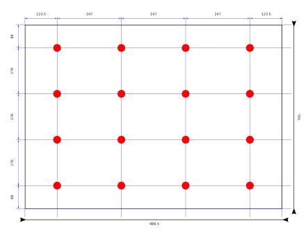
Figure 2: Layout of cameras (distances in cm)
