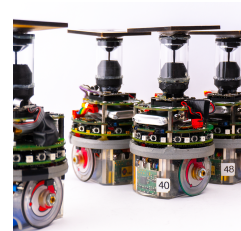
Figure 1: The e-puck robot, a swarm robotics platform of widespread use for research purposes.
