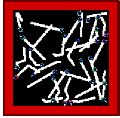
Figure 15: The amount of work performed visualized as the regions of the space that have been visited. ARGoS simulation.
