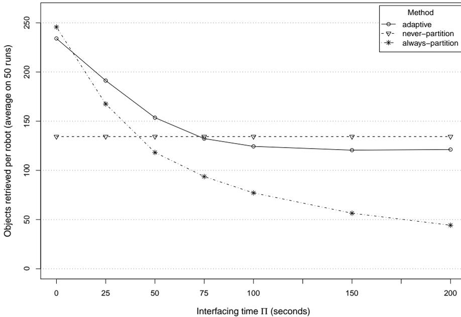
Figure 7: Average amount of objects retrieved per robot at the end of the experiment for different values of the interfacing time  $\Pi$ . The same plot, also reporting the 95% confidence intervals (omitted for clarity here), can be found online (see Pini et al. (2011b)).
