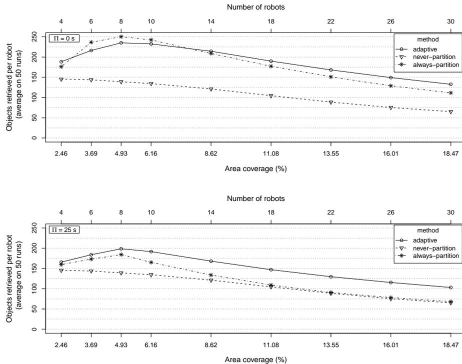
Figure 11: Results of the scalability experiment for  $\Pi = 0$  s (top) and  $\Pi = 25$  s (bottom). The plots report, for each of the three methods, the average individual performance for different area coverages (the top axis reports the corresponding number of robots). The same plot, also reporting the 95% confidence intervals (omitted for clarity here), can be found online (see Pini et al. (2011b)).
