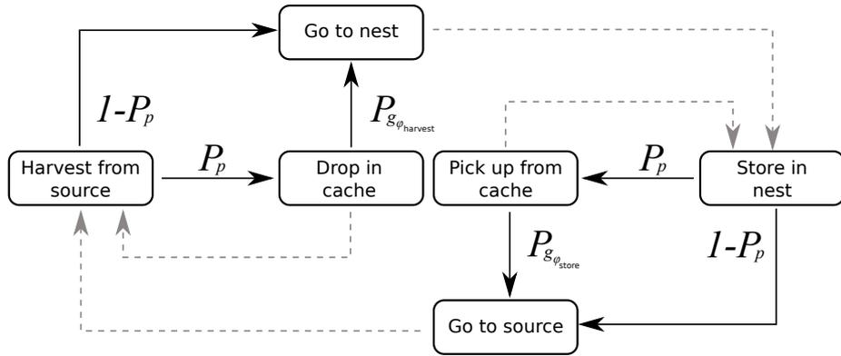
Figure 3: Finite state machine describing the behavior of each robot. The black continuous arcs marked with a label represent stochastic choices that a robot can make.  $P_p$  is the probability of employing task partitioning.  $P_{g_{\varphi_{store}}}$  and  $P_{g_{\varphi_{harvest}}}$  are the probabilities of giving up the store and the harvest sub-tasks respectively (see Section 4 for more details). Dashed gray arcs represent transitions when the robot does not make a choice.
