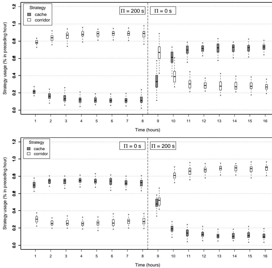
Figure 10: Strategy used in time when the interfacing time  $\Pi$  is varied from 200 s to 0 s (top) and from 0 s to 200 s (bottom). The vertical dashed line marks the instant in which  $\Pi$  is changed (time  $t = 8$  hours and 20 minutes). The total duration of the experiment is divided into windows of 1 hour, each box reports the percentage of usage (over 50 experimental runs) of each strategy in the time window preceding the value reported on the X axis.
