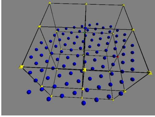
Figure 1: An hexagonal lattice obtained with 100 satellites in the  $xy$  plane of the LHLV frame of the Chief satellite.
