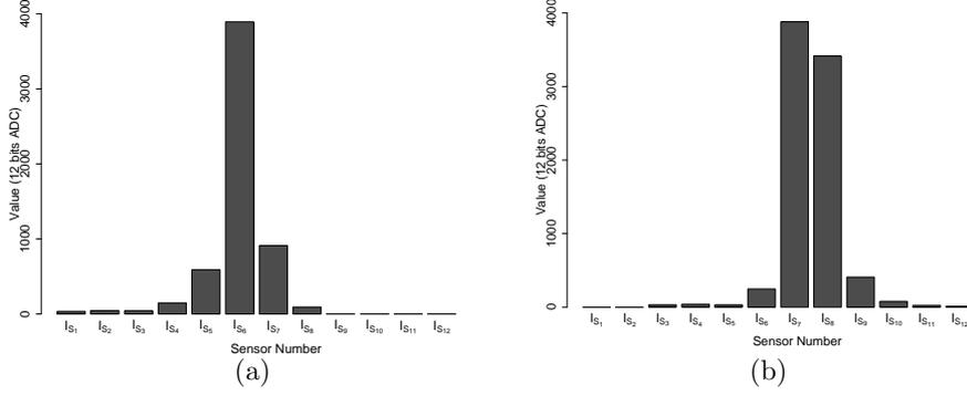
Figure 10: Sensory map for two different reception frames. (a) The emitter is approximately facing a reception sensor. (b) The emitter is in some point in between two reception sensors.
