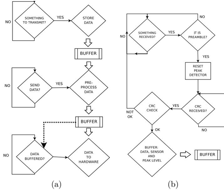
Figure 9: Block diagram of the (a) software emission module and (b) software reception module.
