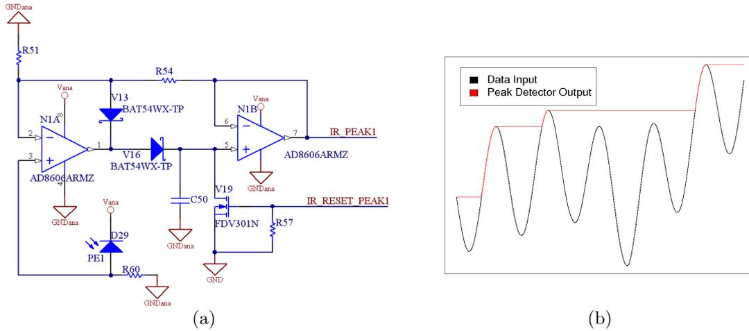
Figure 7: (a) Peak detector functionality. (b) Depiction of one power reception module.
