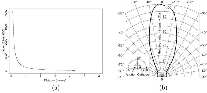
Figure 11: (a) Reception values for different distance transmissions when emitter and receiver sensors are facing each other. (b) Radiation diagram for the PIN diode of the peak detector. (Obtained from the PD100MF0MPx Datasheet).
