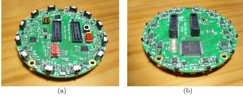
Figure 1: (a) Top and (b) bottom view of the localisation and local communication board.
