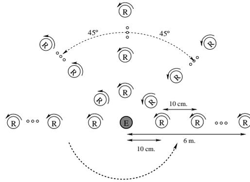
Figure 14: Physical arrangement of the boards for the experiments.
