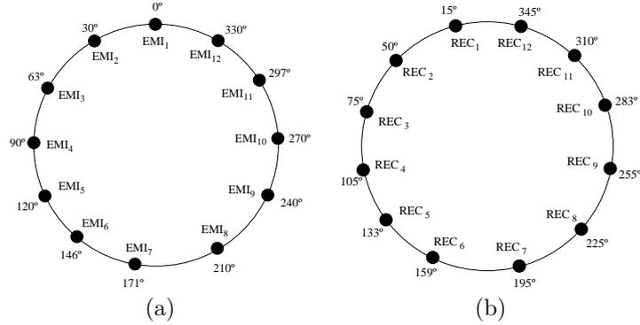
Figure 2: (a) Emitters and (b) Receivers distribution around the perimeter of the board.
