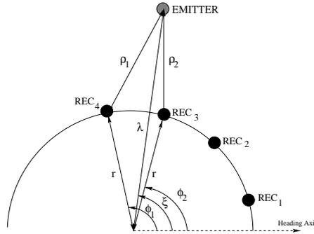
Figure 13: Reception diagram for a specific location and its distance to the different sensors.
