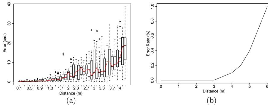
Figure 16: (a) Standard deviation of the distance calculations respect to the real range. (b) Error rate of the communication system.
