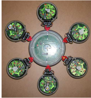
Fig. 5. Experimental setup. An object has to be transported towards a target (on the bottom; not shown). Six robot are manually attached to the object. While some robots are fully operational, others are not capable of perceiving the target.
