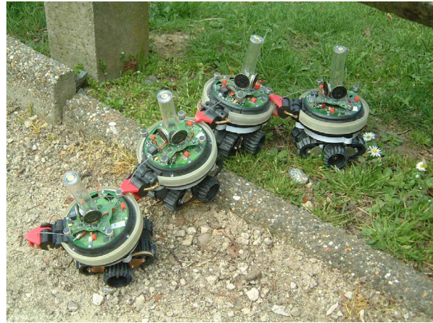
Figure 2. A swarm-bot with a linear shape composed of four s-bots and moving on rough terrain.
