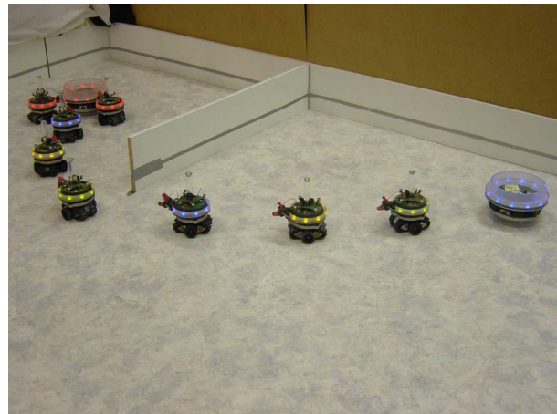
Figure 10. A chain of five s-bots connect the red object on the left to the target location (represented by the blue s-toy on the right). Two s-bots have reached the red object and are preparing to transport it to the target location.
