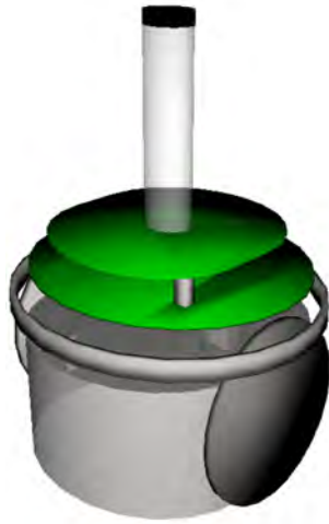
Figure 3.4: A minimalistic simulated e-puck robot modeled in SketchUp.
