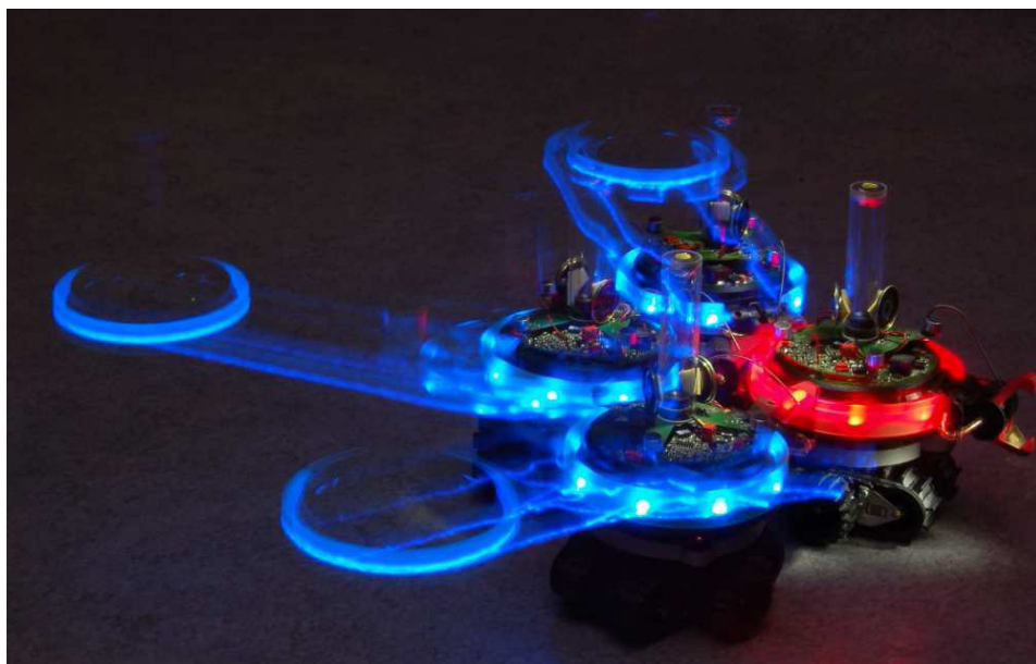
Figure 1.2: A group of s-bots performing self-assembly. The s-bot is the robot platform used in this thesis. The image was exposed during approximately 37sec. In this way the image can show the movement of three robots while attempting to form a physical connection with the robot on the right.
