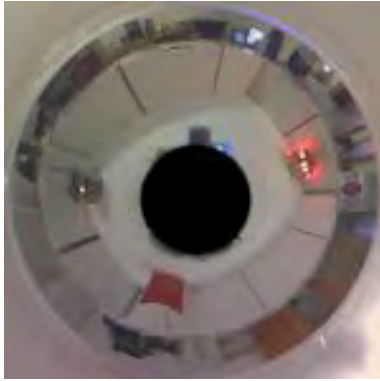
Figure A.3: Snapshot from the omnidirectional camera of an e-puck. Cameras of this type have the advantage that the robot can directly compute distances from the captured image.
