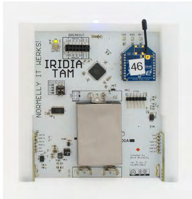
Figure 5.4: Photo of the electronics on the back face of the TAM. At the top right, the 2.4 GHz IEEE 802.15.4 mesh networking module. At the top left, the connector that provides an interface for extending the TAM. At the bottom center, the lithium-ion battery, the same type of battery that is used for the e-puck robot.
