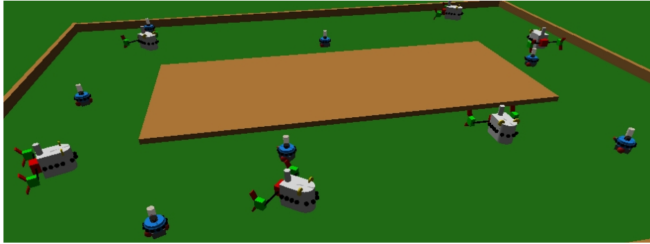
Figure 5.3: Setup for the heavy board lift experiment. A group of hand-bots and a group of foot-bots are in the arena. The foot-bots have to move the hand-bots close to the board, the hand-bot have to collectively lift it.
