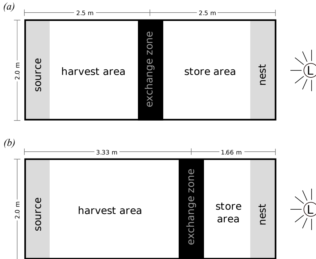
Figure 5.4: Depiction of the environments used in the abstract experiment. (a) Symmetric environment used in the first experiment. (b) Asymmetric environment used in the second experiment. The gray stripes are the source (left), and the nest (right), each 0.5 m deep. The black stripe is the exchange zone, that is 1 m deep. The light source is marked with “L”.
