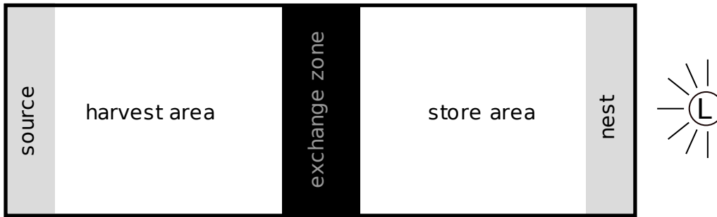
Figure 5.2: General representation of the environments used for studying the sequential task allocation problem. Prey objects are transported from the source on the left to the nest on the right (gray stripes). The robots hand over the objects in the exchange zone (black stripe). The light source is marked with “L”.
