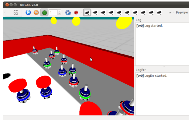
Figure 3.6: The ARGoS simulator running a collective foraging system in a arena delimited by red walls. The gray floor represent the nest, the yellow spots represent lights, the red spots represent prey that the robots transport and the black spots represent prey that are not retrieved yet.
