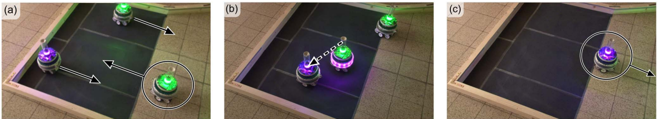
Fig. 7. Illustration of the observation and decision process shown on the example of a single robot. (a) Robot with opinion A (encircled) enters the observation zone. (b) Robot observes another robot with opinion B (the robot shows this to the experimenter by flashing its LED ring) and stores the observation in its memory. (c) Robot leaves the observation zone and the application of the k -unanimity rule changes its opinion to B .
