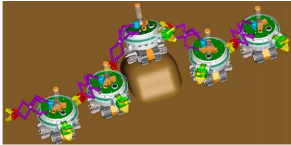
Figure 9. Graphic visualization of how lateral semi-flexible connections are going to be used to keep relative mobility between s-bots while they are in a swarm-bot configuration. This flexible structure can help for instance to pass local small obstacles.
