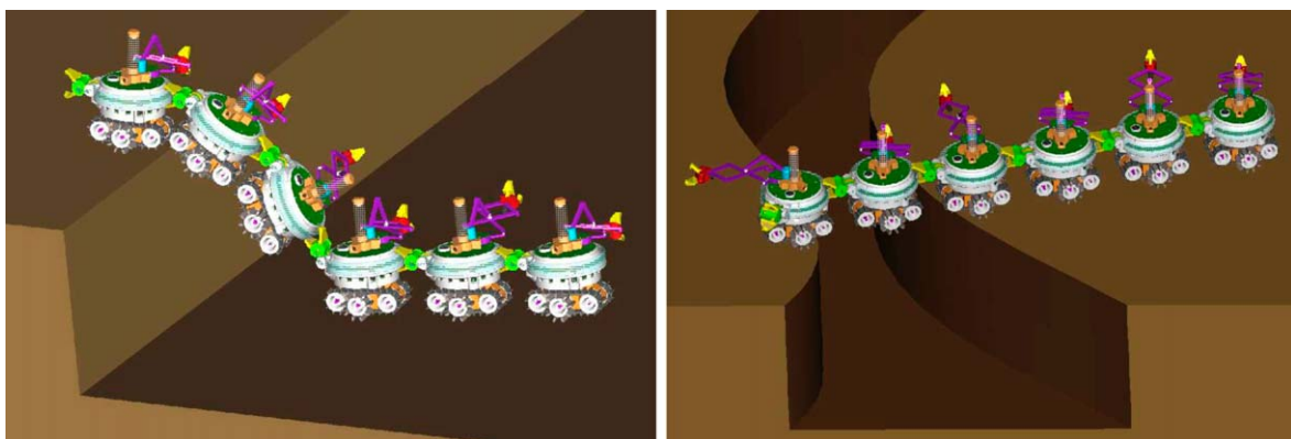
Figure 2. Graphic visualization of how the rigid gripper can be used to connect in a secure way s-bots among themselves so to form chains for overcoming large obstacles or holes.
