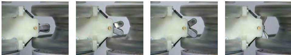
Figure 4.4: From left to right: the gripper of a marXbot opens inside the ring of another marXbot. The mechanism allows the marXbots to connect to each other and form multi-robot structures.
