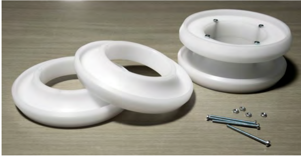
Figure 4.6: Components of the the plastic ring of the object (left) and the plastic ring assembled (right).
