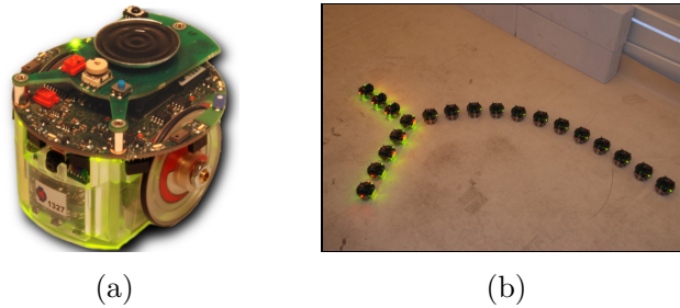
Figure 6.2: (a) The e-puck robot. (b) A swarm of 20 e-pucks arranged in a long and a short path for the setup with resources at different distances.
