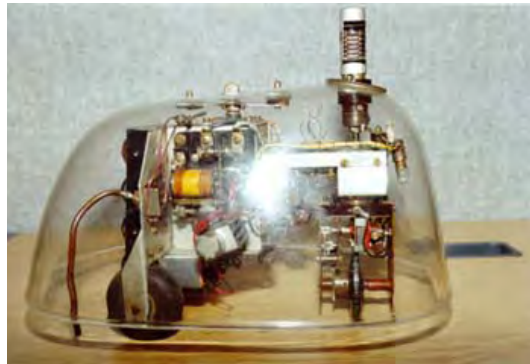
Figure 2.3: One of the turtle robot used by Grey Walter in his studies (restored version shown here).
