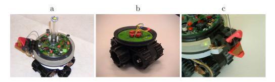
Figure 1.3: (a) A s-bot; (b) the traction system of a s-bot; (c) the s-bot's gripper.
