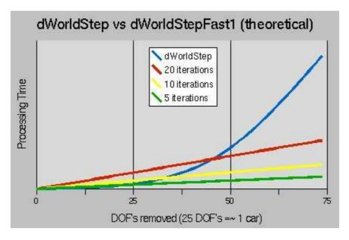
Figure 2.1: Speed advantage of Quickstep [ode doc]
