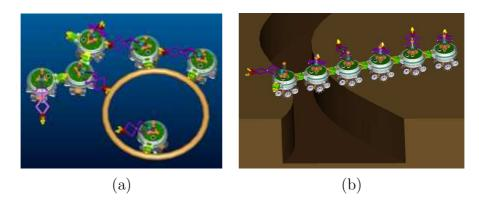
Figure 1.2: Graphical visualization of possible scenarios involving a swarmbot. (a) Retrieving a circular object. (b) Passing over a trough.
