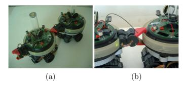
Figure 1.4: (a) Two connected s-bots; (b) detailed view of a connection between two s-bots
