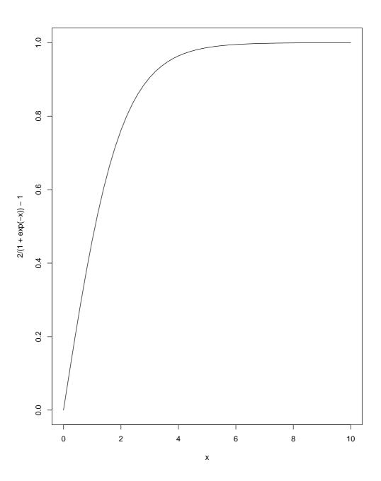
Figure 3.2: Sigmoidal saturation function
