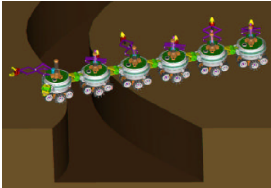
Figure 4: Robots in rigid formation can overcome small holes.
