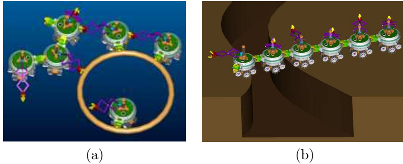
Figure 1.2: Graphical visualization of possible scenarios involving a swarm-bot . (a) Retrieving a circular object. (b) Passing over a trough.
